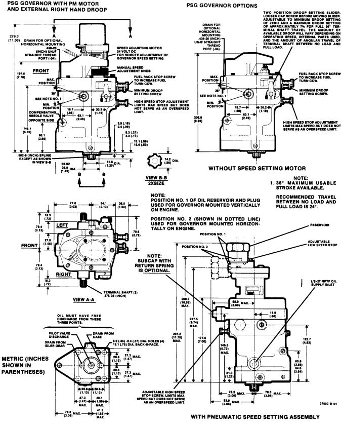
OUTLINE DRAWINGS OF CAST IRON CASE PSG GOVERNORS (DO NOT USE FOR CONSTRUCTION) METRIC (INCHES SHOWN IN PARENTHESES)
